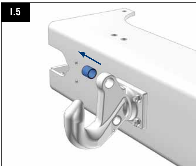
Demontage der oberen Lagerbuchse Dismantling of the upper bearing bushing
