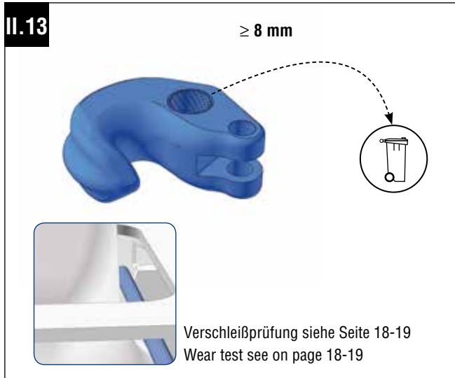
Demontage (Kuppelhaken-) Lagerbuchsen verschlissen Dismantling of the bearing bushing (coupling hook) worn
