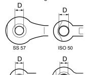
The wear limits for the bushing/wear ring in the drawbar eye are indicated in table.
