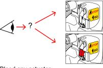
Bleed any actuator. Check that there is slight axial play in the coupling bolt using a mandrel. (The closing spring tension must be overcome.)
