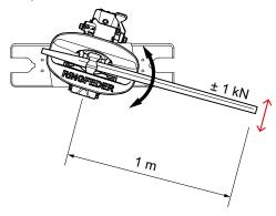
The coupling should rotate at 1,000 Nm.
