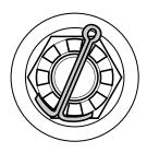
The castellated nut must be torque-tightened using torque. The cotter must be properly locked.
