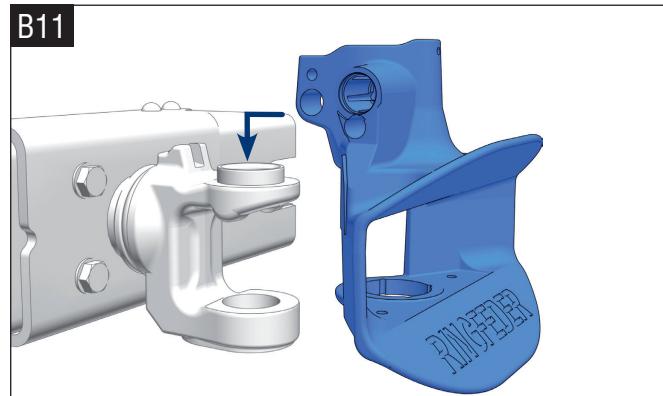
Fitting of the coupling assembly
